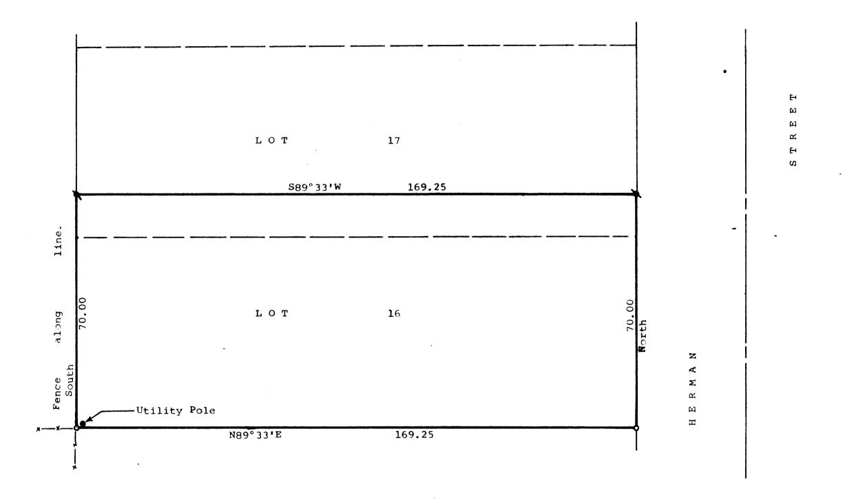
Scale - 1'' = 20'o = 3/4" Dia. Iron Pipe Found 🔪 = 🧏 Dia. Iron Pipe Found **1**→ = Fence Line
